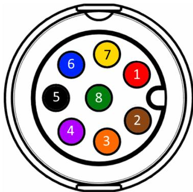
GPIO connector as seen from rear Atlas view. Pin colors correspond to GPIO-M8 cable from Lucid Vision Labs.
