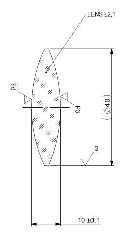
YAG-BBAR R(ABS) < 0,25% @ 532nm @ 0° AOI R(ABS) < 0,25% @ 1064nm @ 0° AOI R(AVG) < 1,0% FROM 500-1100nm @ 0° AOI
