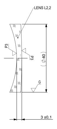
YAG-BBAR R(ABS) < 0,25% @ 532nm @ 0° AOI R(ABS) < 0,25% @ 1064nm @ 0° AOI R(AVG) < 1,0% FROM 500-1100nm @ 0° AOI
