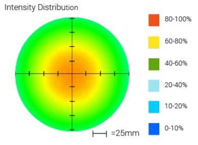
Optical measurement taken using DF198-180WHII3 @ 100mm
