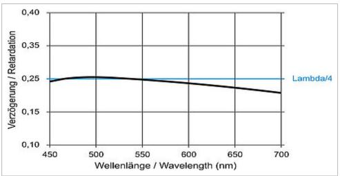
The WP140HE is a highly transparent optical retarder with a quarter-wave retardance for 560nm. The achromatic properties of the polymer film based on polycarbonate allows the use of the quarter-wave sheet within the range 450-650nm.
