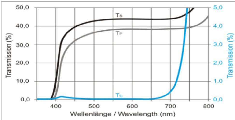
The XP44 is an optimized sheet polarizer offering the highest possible light transmission. The polarizer distinguishes itself through its excellent polarization within the visible region absorption spectrum of 400-700nm. This filter is typically used for applications where maximum light transmission is required.
