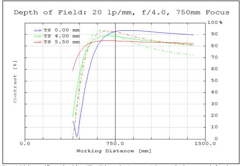
Figure 6: Polychromatic diffraction through-focus MTF at 20 linepairs/mm (image space). Contrast is plotted to two times the focus distance.
