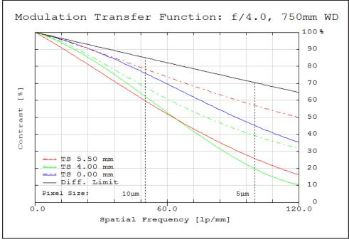
Figure 5: Image space polychromatic diffraction FFT Modulation Transfer Function (MTF) for λ = 486nm to 656nm. Included are the Tangential and Sagittal values for field points on center, at 70% of full field and the maximum sensor format. Solid black line indicates diffraction limit determined by f/#-defined aperture. Frequencies corresponding to the Nyquist resolution limit of pixel sizes are indicated.
