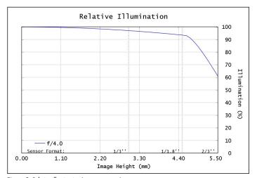
Figure 2: Relative illumination (center to corner)
