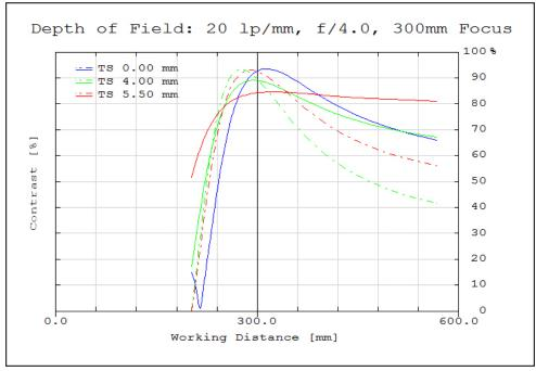
Figure 4: Polychromatic diffraction through-focus MTF at 20 linepairs/mm (image space). Contrast is plotted to two times the focus distance.
