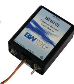
The BPS101 is a low-cost high-performance constant current light source which uses a replaceable Tungsten Halogen bulb rated for 10,000 hours. This device uses a constant current setting which provides precision current control, allowing for stable performance.
