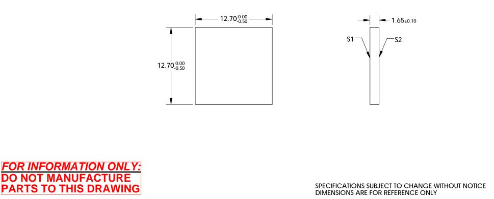
Edmund Optics® S1 S2 PLANO PLANO SHAPE BS POLKA-DOT 70/30 12.7mm SQ THIRD ANGLE 80-50 TITLE 80-50 SURFACE QUALITY PROJECTION 90% 90% CLEAR APERTURE SHEET ALL DIMS IN mm DWG NO **PROTECTIVE AS NEEDED PROTECTIVE AS NEEDED** 47607 BEVEL 1 OF 1
