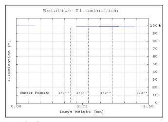
Figure 2: Relative illumination (center to corner)
